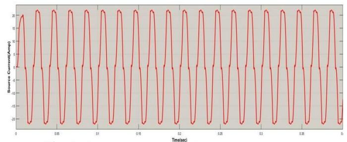
**Fig -7:** Source current waveform without compensation
