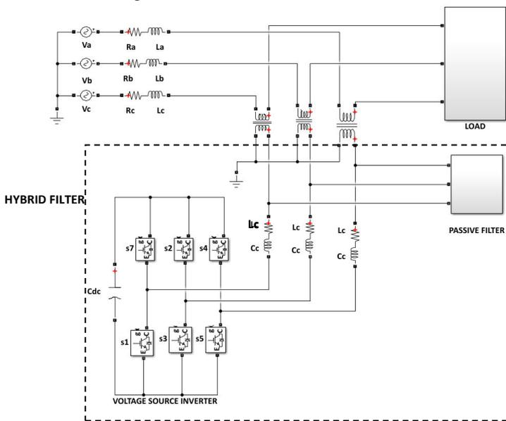
Fig -1: Hybrid Filter With a Combination Of Series Active And Shunt Passive Filter
