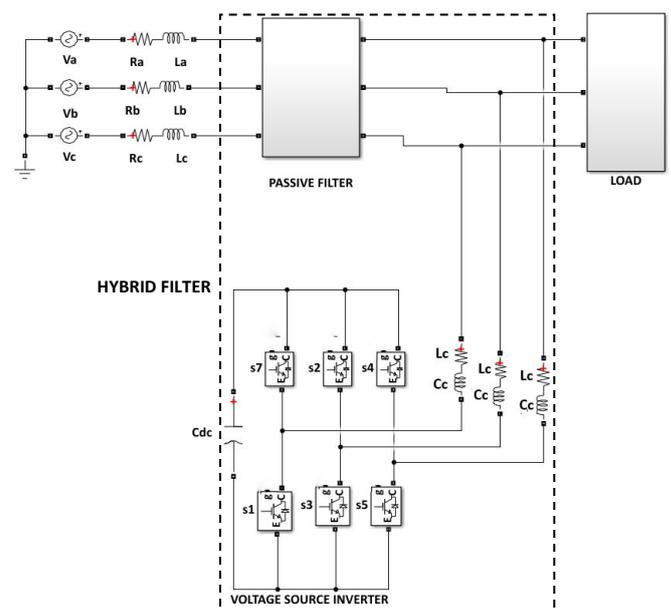
Fig -3: Hybrid Filter With a Combination Of Series Passive And Shunt Active Filter
