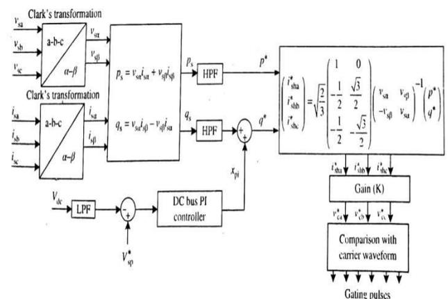
Fig -5: Modified Instantaneous Reactive Power Theory
