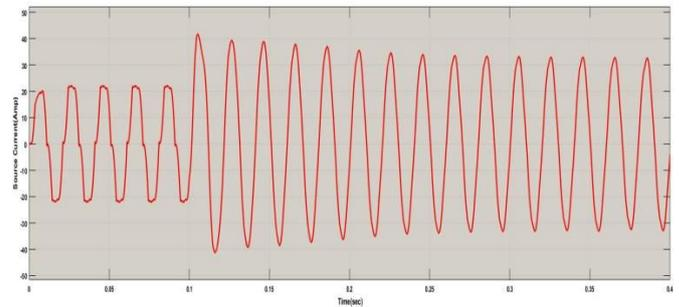
**Fig -12:** Source current waveform with Hybrid active power filter compensation
