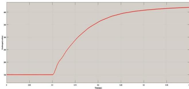
**Fig -16:** DC link capacitor voltage
