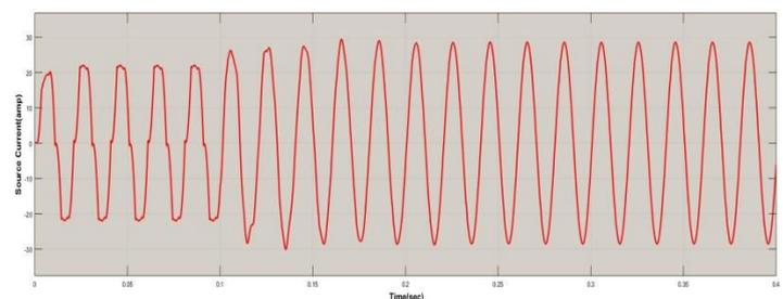
**Fig -8:** Source current waveform with Hybrid active power filter compensation
