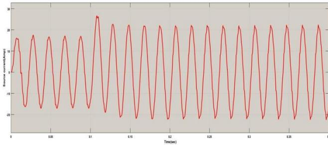
**Fig -15:** Source current waveform with hybrid filter compensation
