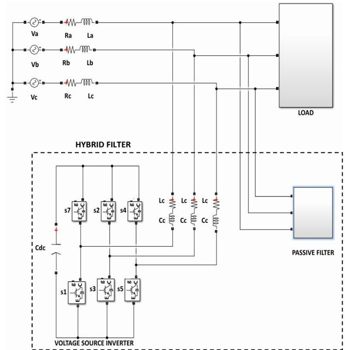
Fig -2: Hybrid Filter With a Combination Of Shunt Active And Shunt Passive Filter
