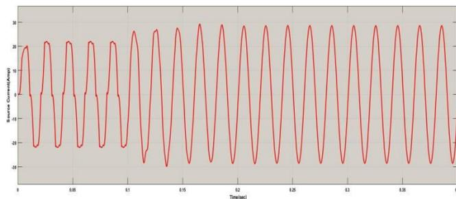
**Fig -10:** Source current waveform with hybrid filter compensation
